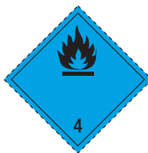
(No. 4.3) Class 4.3 Substances which, in contact with water, emit flammable gases Symbol (flame): black or white. Background: blue. Figure '4' in bottom corner.
