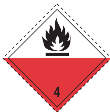
(No. 4.2) Class 4.2 Substances liable to spontaneous combustion Symbol (flame): black. Background: upper half white, lower half red. Figure '4' in bottom corner.
