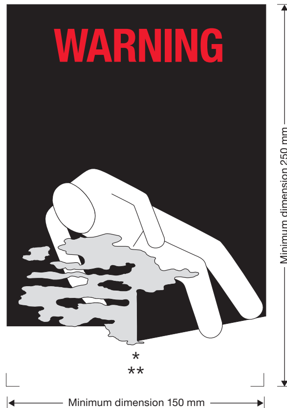
Coolant/conditioning warning mark for cargo transport units
