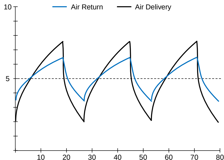
Figure 8.14 Variations of air temperature under thermostatic control
